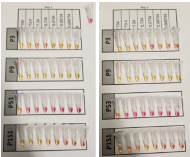
Figure 13: Sensitivity testing of four core primer sets (P3, P9, P53 and P151) using 10-fold dilutions of DNA extracted from Clariireedia spp.
