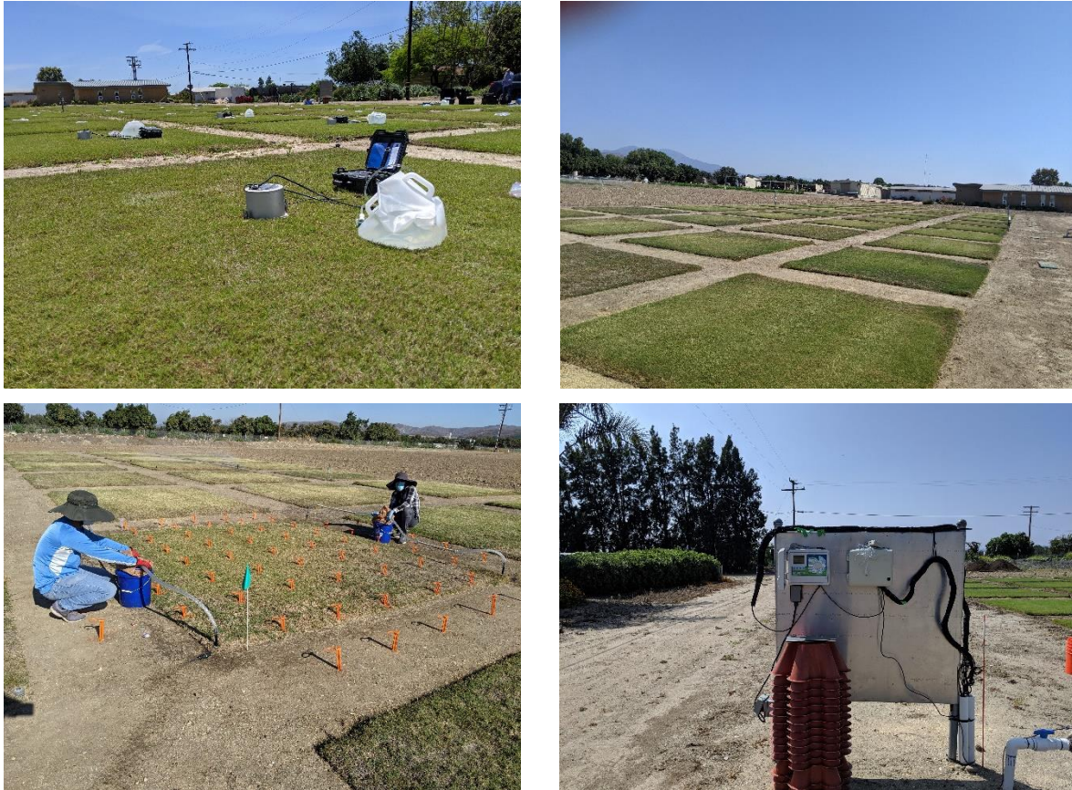
Figure 1. Top: Automated infiltrimeters are being used to measure the potential impact of varying irrigation rates using recycled water on infiltration rate (left). An overview of the research plots (right). Bottom: Graduate students are conducting a flow and catch can test (left). An overview of the smart soil moisture-based irrigation controller used in this study (right).
