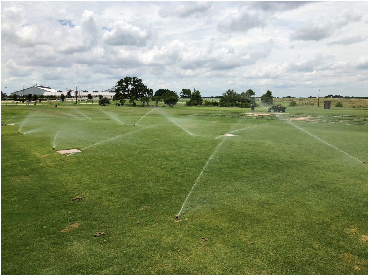
Figure 4. Image of the sand-capping irrigation facility at Texas A&M University, College Station, TX. The facility contains 16 independently irrigated zones and was established in 2018 with Latitude 36 hybrid bermudagrass atop a 7" sand-cap.
