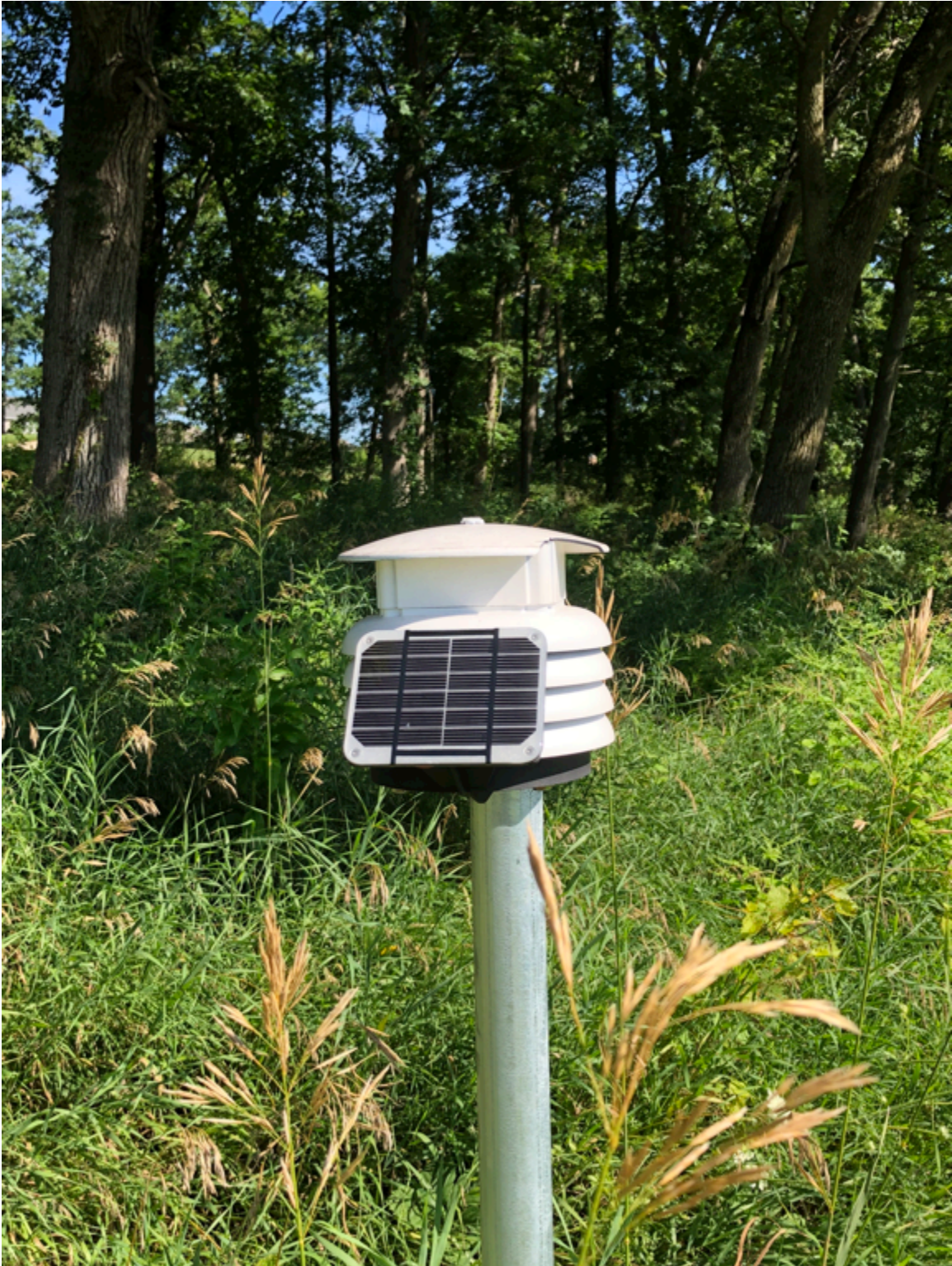
Figure 3. The weather station custom-built by Walker Olson at Toro at the Hole 18 research site. The same sensors were also placed at Hole 7 and the OJ Noer.
