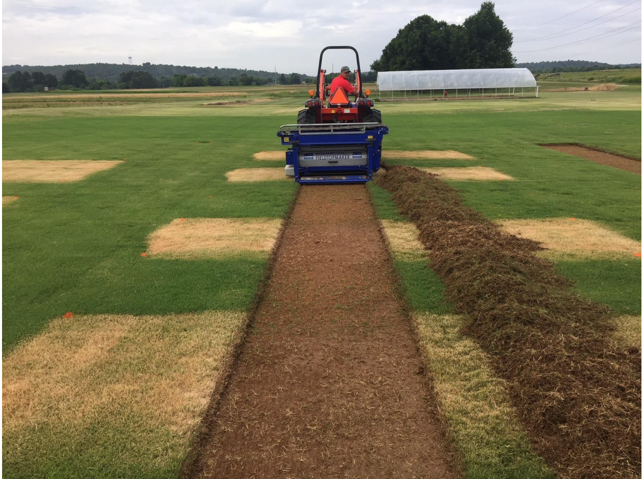
Figure 1. Koro Field Topper being used to fraise mow plots at the Fayetteville Research Station in 2018.
