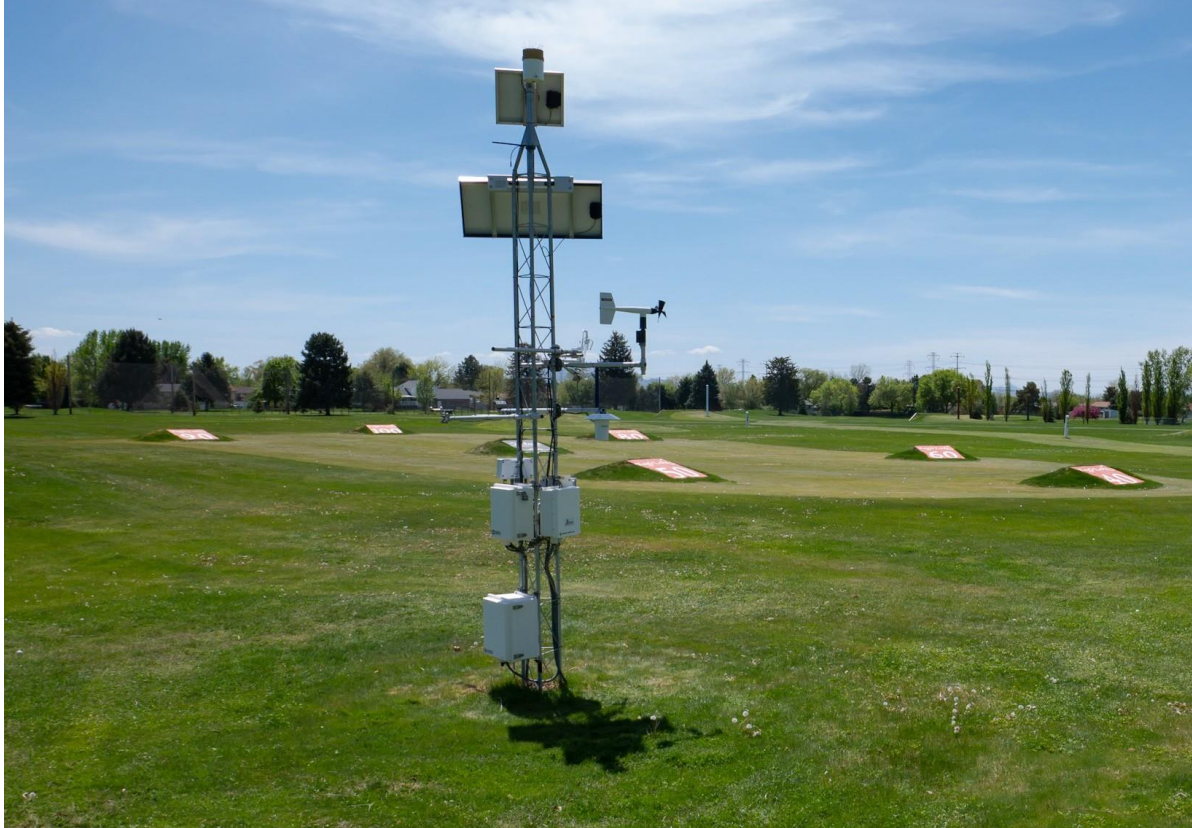
Figure 1. Image of eddy covariance station. The upwind distance “sensed” is about 350 m.
