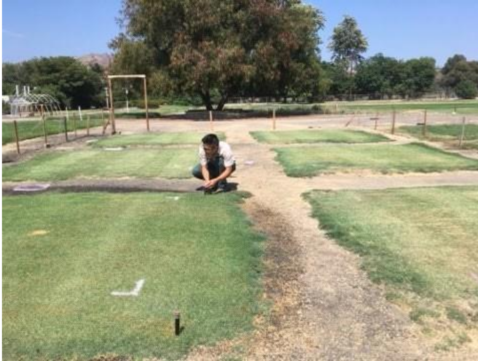
Figure 1. Each plot is individually zoned and has a rotating nozzle sprinkler at each of the four corners.
