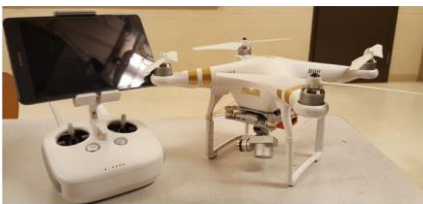
(a) The off-the-shelf DJI P3 UAV with an RGB camera
