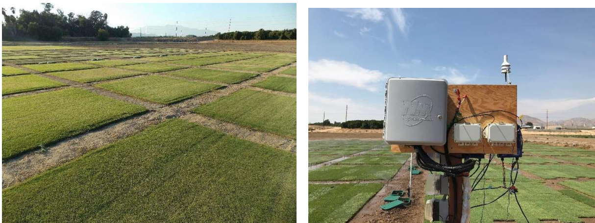
Figure 1. The research plots under tall fescue and bermudagrass turf species (left) and the Weathermatic weather-based smart irrigation controller used to impose irrigation treatments (right).
