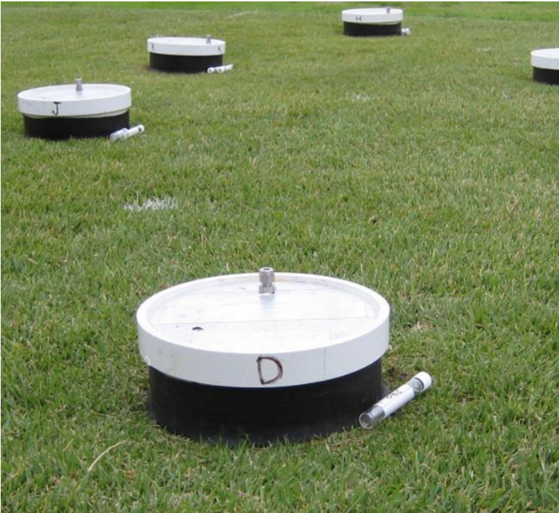
Figure 3. Close-up of one of twelve static chambers used for sampling N 2 O.
