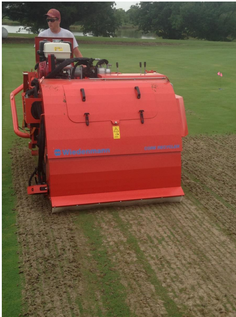
Figure 1. Wiedenmann Core Recycler used to separate sand from organic matter in the top portion of a hollow tine core.
