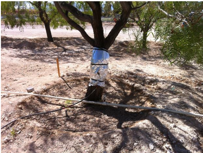
Granier probes installed and covered with protective insulation.
