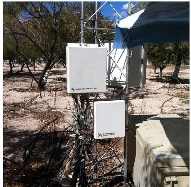
Data logger with cables from 30 granier probes installed in the 10 species (3 replicates).
