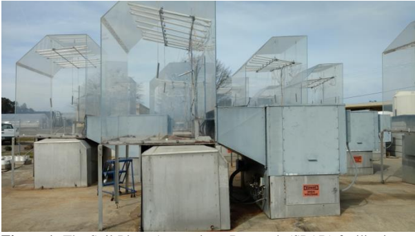
Figure 1: The Soil-Plant-Atmosphere-Research (SPAR) facility is located at Mississippi State University in Starkville, Mississippi. The facility is composed of ten naturally-lit chambers on a 20 \times 30 m concrete pad. Each unit is composed of a Plexiglas chamber measuring 2.5 m high, a steel soil bin measuring 1.0 m deep \times 2.0 m long \times 0.5 m wide, and an air handling unit.
