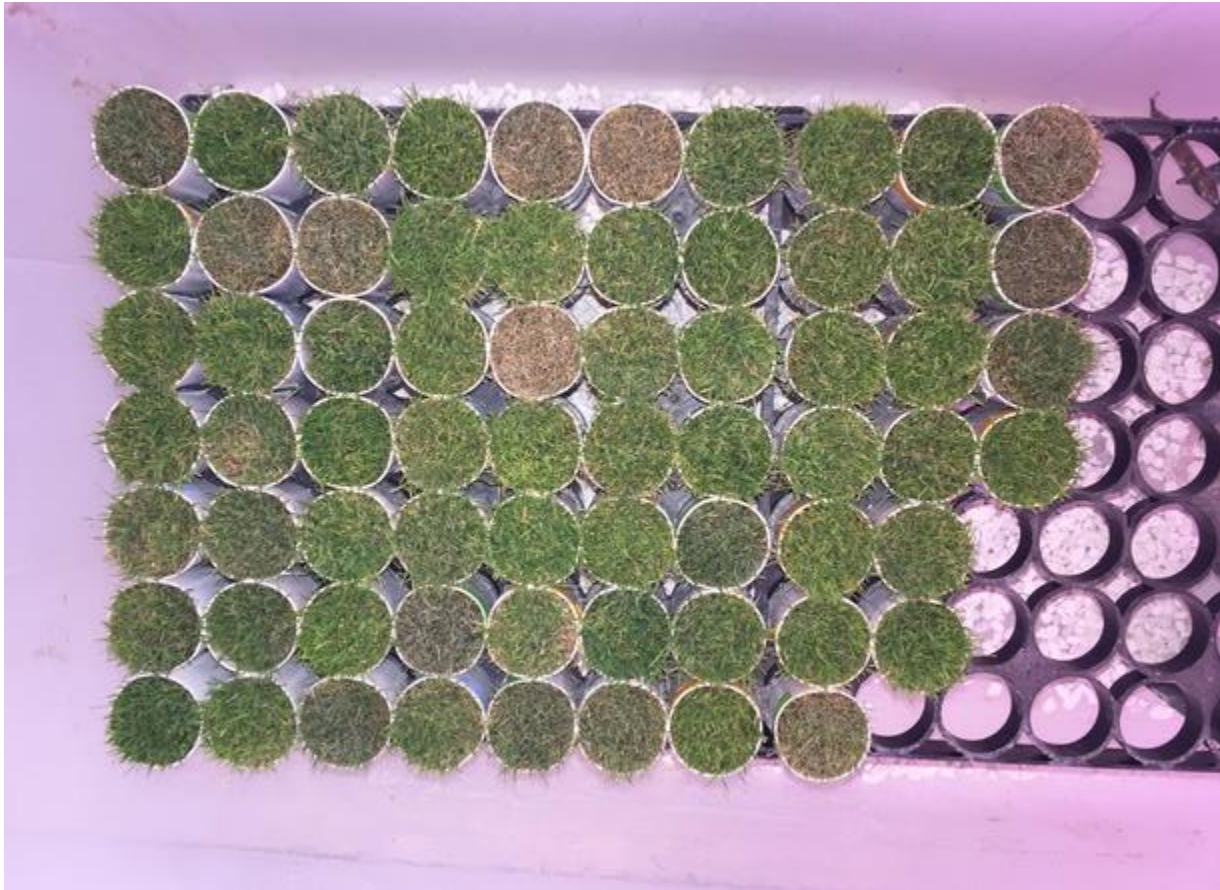
Figure 5. Deficit irrigation treatments are being applied to achieve various crown moisture content ranges. After prolonged deficit irrigation, cones are subjected to decreasing freezing temperatures to evaluate which crown moisture content range provides the greatest level of cold hardiness. Visual water stress and photooxidative stress can be observed in deficit irrigated cones.
