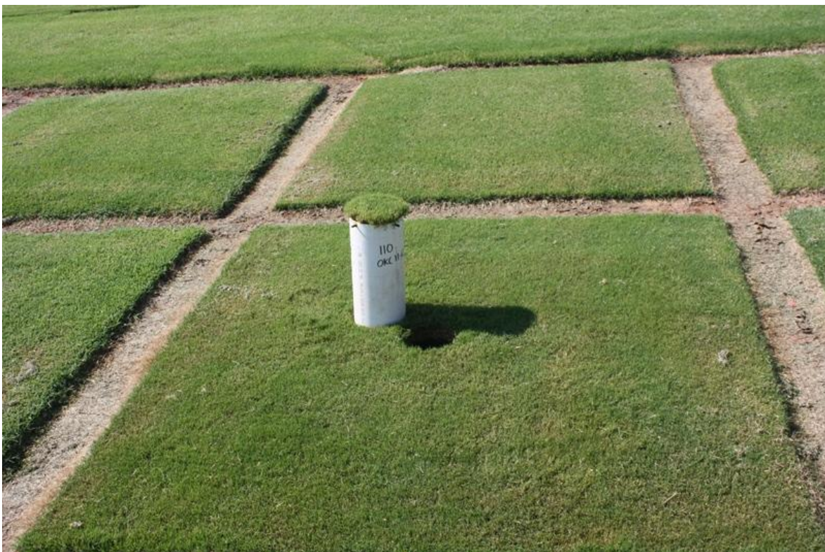
Photo 2. A lysimeter in a field plot.
