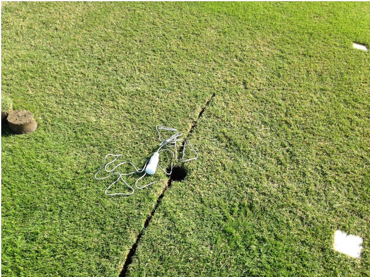
Figures 1. Logging soil temperature probes were installed at the turf crown/soil interface to monitor soil temperatures during the study.
