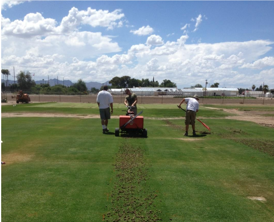
Figure 2. Tillage treatments consisted of one pass with walk-behind aerator outfitted with hollow tines. Soil cores were raked off and removed from the plots.
