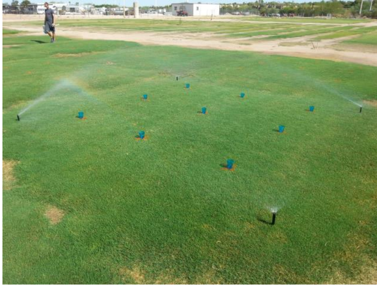
Figure 4. Irrigation treatments consist of a deficit and surplus (leaching) regime. Catch cans are used to monitor the precipitation rates of the plot irrigation systems.
