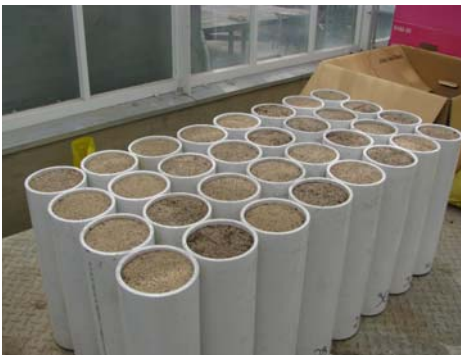
Sand-based profiles (10 cm diameter, 30 cm length) were built to USGA-specifications in PVC columns.
