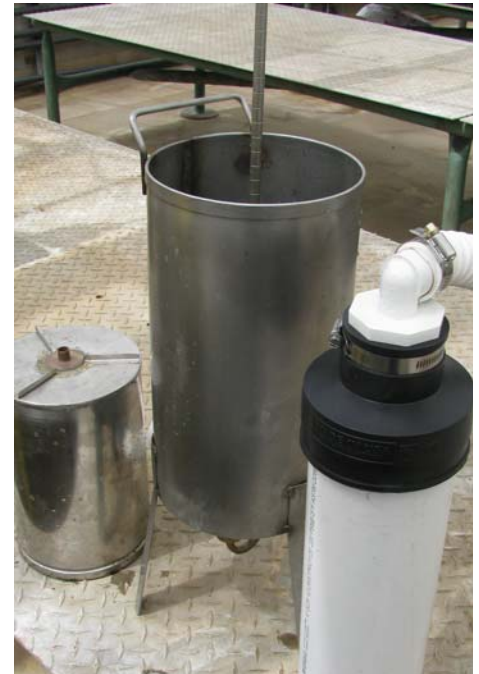
Hydraulic conductivity will be measured using an automated falling head permeameter.
