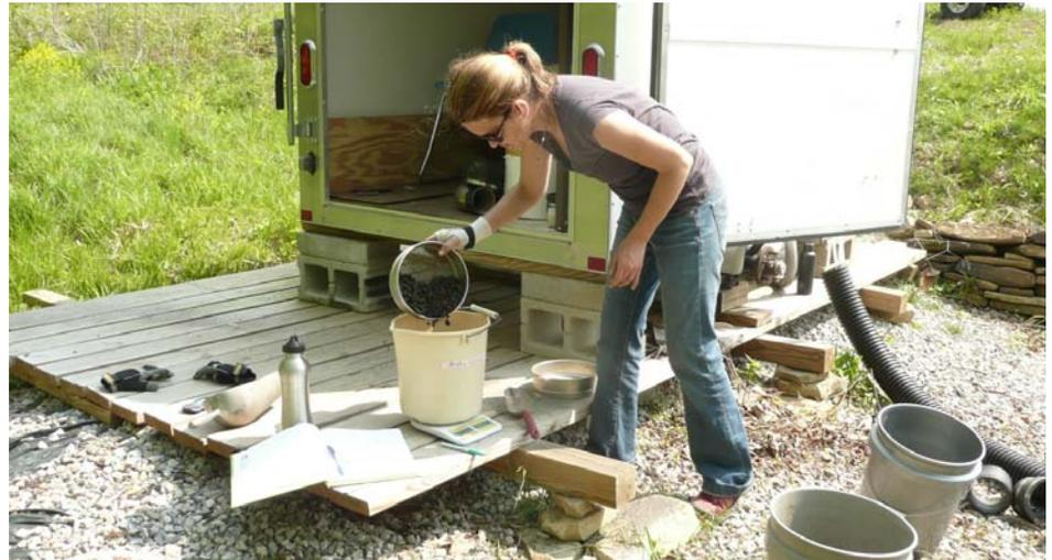
Each tile was filled with 28.5 kg of steel slag that was previously removed of fines with a U.S. Standard Mesh #16, 18 mm sieve.
