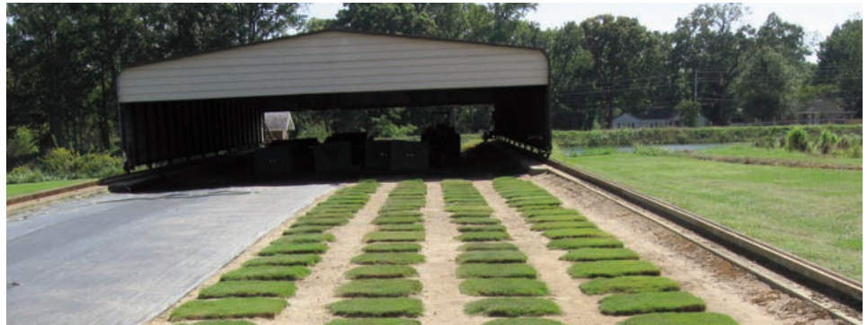
Automated rain-out-shelter covers field plots during natural rainfall events allowing us to impose drought conditions.
