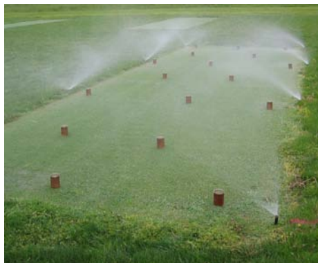
The irrigation system was calibrated with cans to ensure that water was uniformly distributed across each 5 ft x 10 ft subplot.
