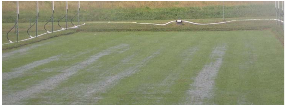
Development of "streams of flow" are seen in large plots midway through a simulation rainfall event.
