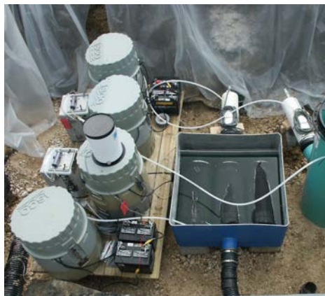
In late 2005, the field site was instrumented with the two distinct commercial filters and automated water samplers.
