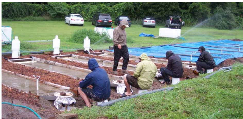
A runoff plot, consisting of 12 vegetative filter strips (VFS, 4.6m x 0.09 m), has been established at the UMASS Turfgrass Research Center, South Deerfield, MA.
