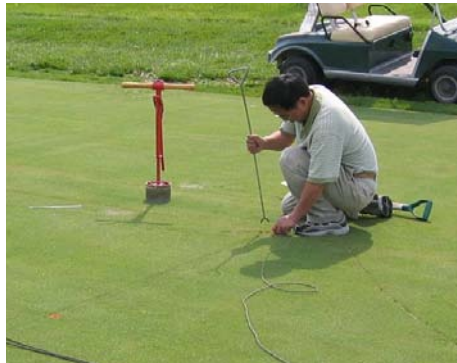
Soil temperature was measured by installing temperature sensors about 0.8 inches below the soil surface.
