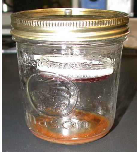
The Illinois Soil Nitrogen Test (ISNT) involves heating soil in a basic solution that converts the amino sugar into ammonia. The ammonia is absorbed by a boric acid indicator solution. The boric acid solution is titrated to measure the ammonium that gives the relative amount of amino sugar in the soil.
