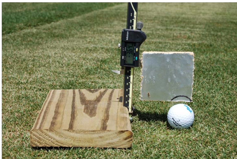
Treatments with Primo or Primo + Cutlass were the most effective for preventing the golf ball from sinking into the 'TifSport' turf. Nitrogen level by itself appeared to have little effect on ball lie.
