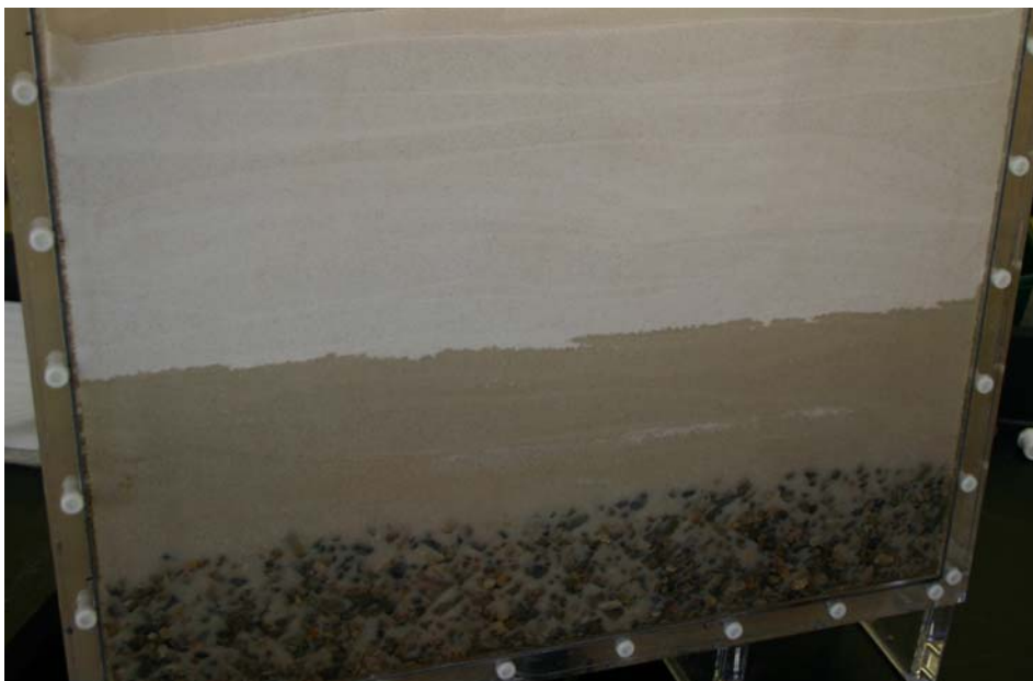
Sand rootzone water movement will be conducted on a larger scale in translucent acrylic viewing boxes. Questions such as "What happens to water flow if sand migrates into the gravel layer during construction?" can be addressed with these boxes.
