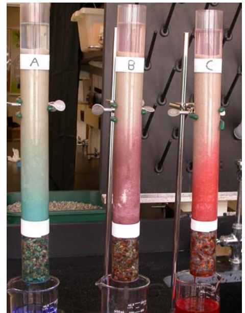
Various tracker dyes (top) are being used to demonstrate water movement in unsaturated sands. The tracker dyes clearly demonstrate the zone of saturation that develops at the interface of the sand-gravel rootzone system (below).
