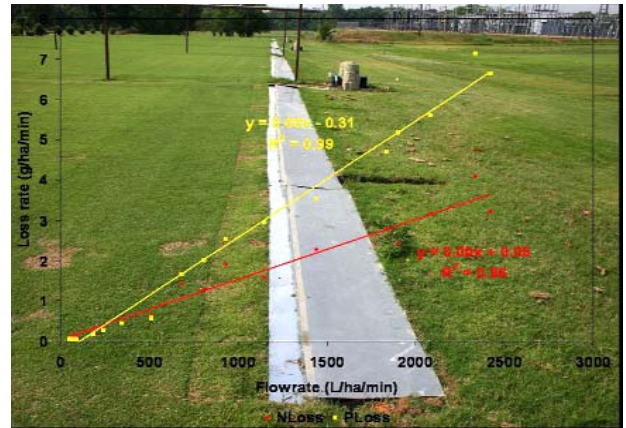
Figure 2. The relationships between mean nitrogen and phosphorus loss rates and natural rainfall runoff flow rates averaged over events after categorizing by time after the initiation of runoff.
