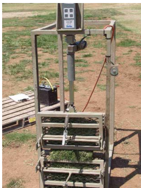
Sod tensile strength is a critical component of sod production and handling characteristics. Show here is a machine that tests for sod tensile strength (shear strength).
