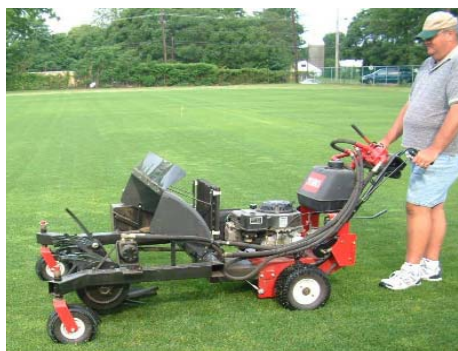
A wear simulator was developed to identify improved wear tolerance in Kentucky bluegrass and bentgrasses.
