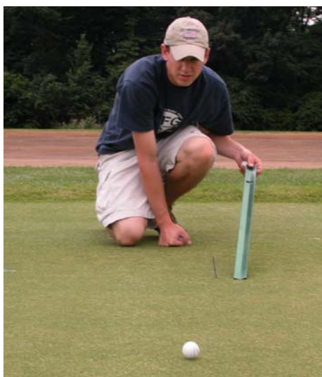
Lightweight rolling every other day slightly reduced anthracnose and increased ball roll distance.
