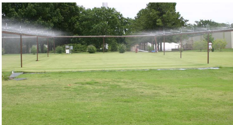
Time domain reflectometers and irrigation were used to maintain soil moisture at field capacity throughout the study.
