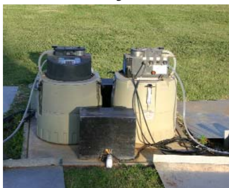
Collectors were programmed to collect runoff samples at 5-min intervals any time runoff occurred.
