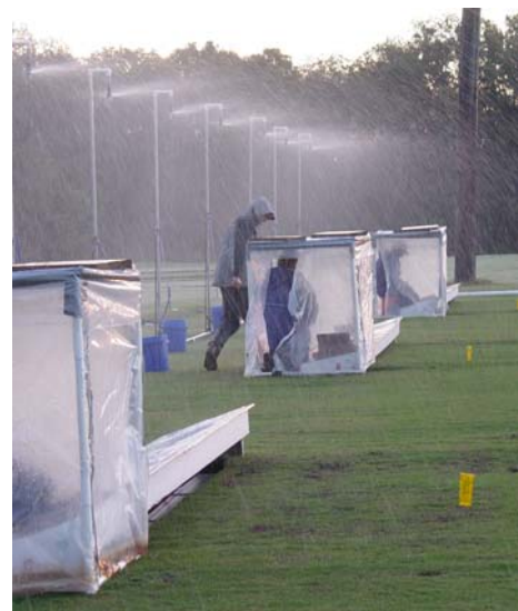
A rainfall simulator was constructed to generate runoff from each of the turfgrass plots
