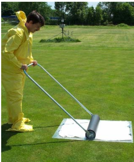
Collecting dislodgeable foliar residues (DFR) with the California roller (CA roller). The 32-lb roller is slowly rolled over a 6 ft 2 cloth 10 times. Pesticide residues transferred to the cloth are considered dislodgeable.
