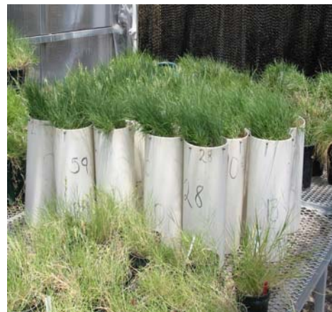
Weighing lysimeters allow for precise volumetric water content and water use determination.
