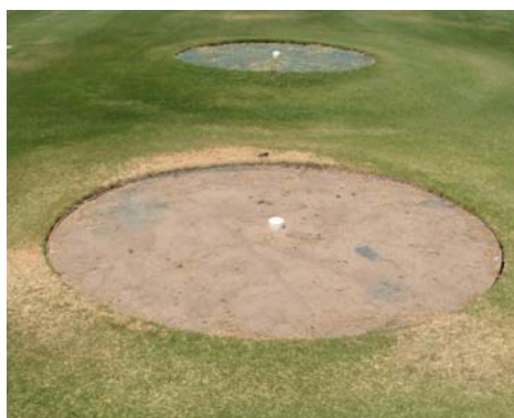
Large monolith lysimeters were transplanted to 'Tifway' bermudagrass and 'AZ 138' saltgrass to compare evapotranspiration rates (water use).
