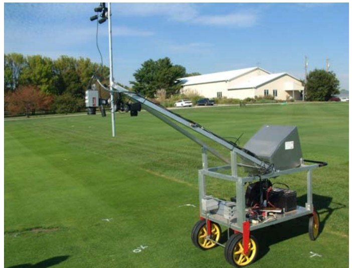
Using specially designed equipment to record turfgrass quality parameters could eliminate the variation inherent among human evaluations.
