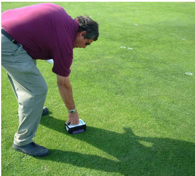
At the University of Illinois, Dr. Tom Fermanian is studying equipment to measure percent living cover, genetic color, leaf texture and other parameters in an effort to eliminate subjective human evaluations.
