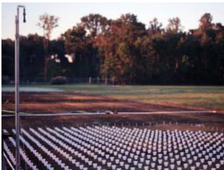
Over the summer, an extensive evaluation of the distribution pattern for the rainfall simulator was performed by conducting several individual sprinkler head audits.
