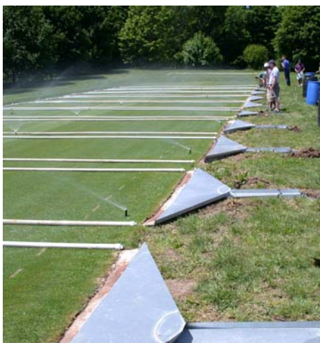
The experimental area has a 5% downward slope and individual runoff plots are 10 by 30 ft.
