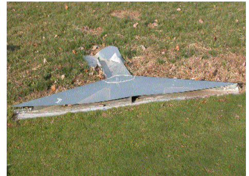
At the base of each plot is a collection flume that funnels runoff into a small pit.
