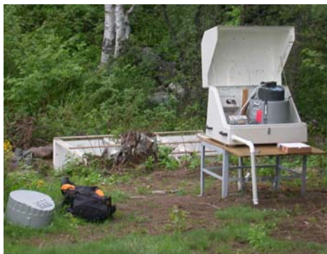
Two ISCO 6712 automatic collection systems were installed at the site in April of 2003 when sampling began.
