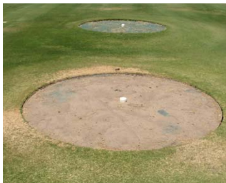
Large monolith lysimeters were transplanted to Tifway bermudagrass and to AZ 138 saltgrass to compare evapotranspiration rates (water use).
