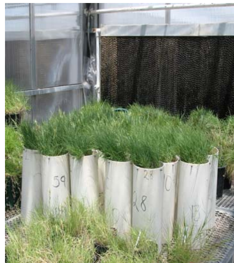
Weighing lysimeters allow for precise volumetric water content determination and subsequent water use.
