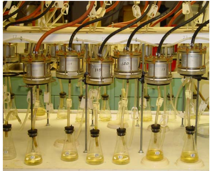
In the lab, this apparatus is used to measure the infiltration rate of cores collected in the field.
