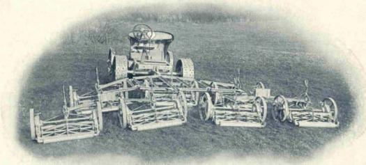
1932 MODEL WORTHINGTON "MULTIGANG" When drawn by a Worthington lawn tractor this Multigang (the greatest achievement in lawn mowing machinery) cuts an acre in four minutes or 18 holes in five hours.
