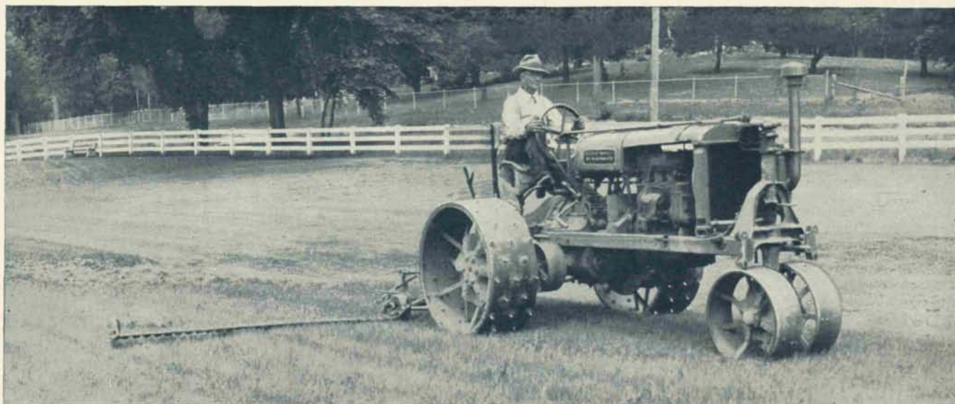
The McCormick-Deering Fairway Tractor with 7-ft. built-in power mower, cutting the rough on the Edgebrook Golf Course, Rockford, Ill. Mr. Rudelius is on the Fairway
