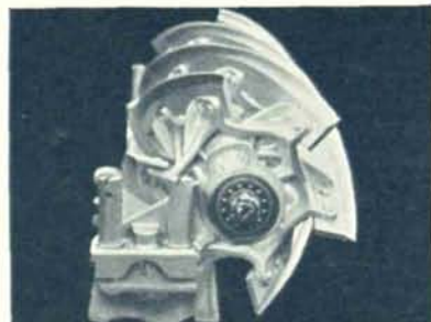
Single unit reel and bed knife bar assembly.
