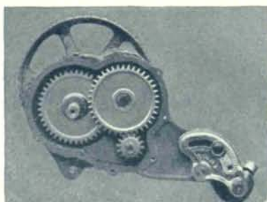
Sliding pinion throwout disengaging gears.
