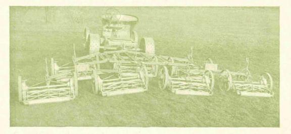
The Worthington Convertible Multigang having seven units arranged in two rows, cutting a swath of sixteen feet. In combination with a Worthington tractor, this wonderful apparatus will cut an acre of grass in four minutes.
