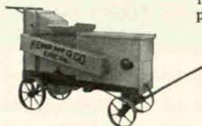
No. 1 Gasoline Model. Handles 6 cu. yds. per hr. Another larger size, gas or electric, handles 12 cu. yds. per hr.
