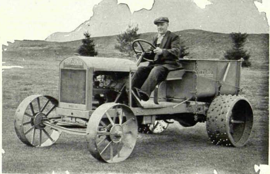
The new Toro Junior Model B-30 has a wheel base of 98 inches, and is equipped with a dump box. Exhaustive field tests have proven that the new Toro will climb a 30% grade with a full body load. Note the trim appearance and well balanced lines.
