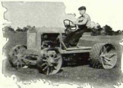
Graceful lines and extreme flexibility are among the dominant features of the new Toro Junior Tractor. Standard equipment includes self-starter, generator, battery and full length muffler, insuring quiet operation.
