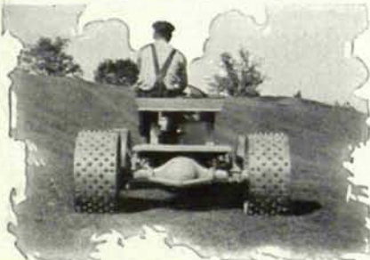
The sturdy bevel gear rear axle will transmit full possible drawbar horsepower. Pulling out the rear end, a fault common to most of the present day small tractors, is absolutely eliminated in the new Toro.
