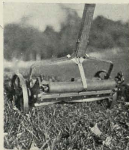
Special lifting attachment for all side wheel mowers, a new specialty of the Stumpp & Walter Co.
