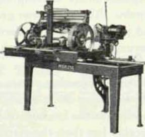
Grinds all type of power-driven, fairway, putting green and hand mowers without removing mower wheels or reel knives. Carriage has travel of 42 inches. Very fast and extremely accurate. 6-inch grinding wheel driven by 1/2-h. p. motor and V belt. Very quiet running.
