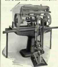
Sharpens quickly and accurately the bed knives and reels of all mowers.
