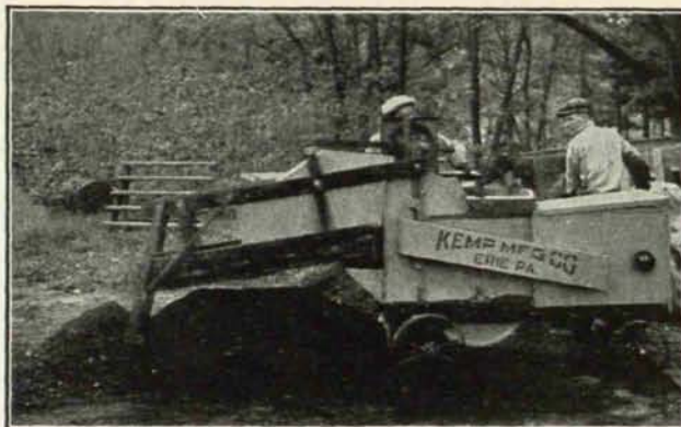
Shredding and screening soil in one operation on a well-known golf course
