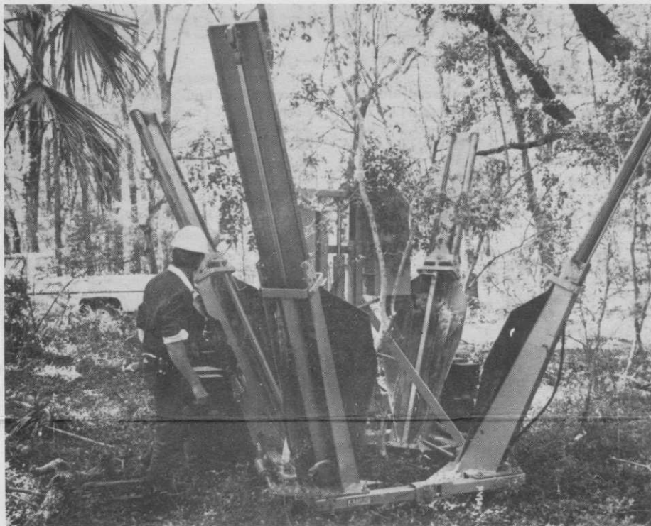
This hydraulic-powered tree spade is transplanting trees for future use on the new golf course under construction on remote Daufuskie Island.
