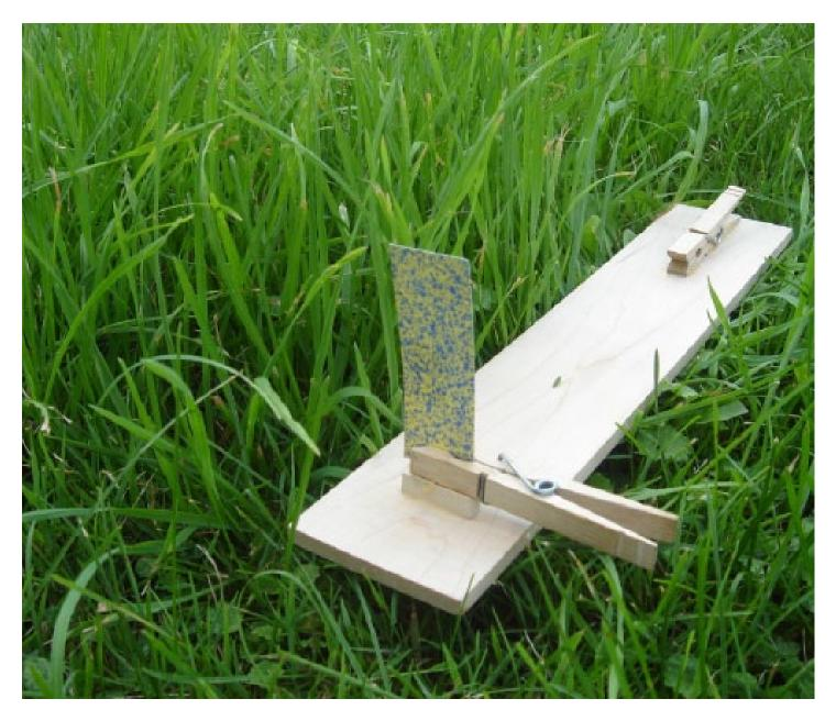
to demonstrate with WSP. Simply clip two WSP's taped back-to-back to a base and orient them vertically like a blade of grass. Align the WSP perpendicular to the direction of travel. Spray over them with a flat fan nozzle and compare the coverage on the front WSP to the back. Repeat the test using a twinfan nozzle and you should note more coverage on the back WSP
