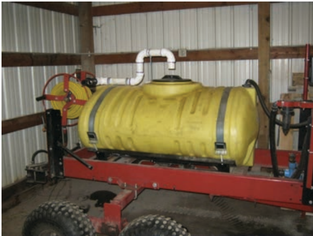
Fixed ridged air gap
