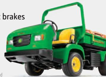
\*Payload includes 200lb (90.7kg) operator, 200lb (90.7) passenger and loaded attachment, 2WD with Heavy Duty Suspension, Wide Rear Tire & 4-Post ROPS. Payload tested in accordance with ANSI / ITSDF B56.8 – 2006 standard. ROPS tested in accordance with ISO 21299-2005.
