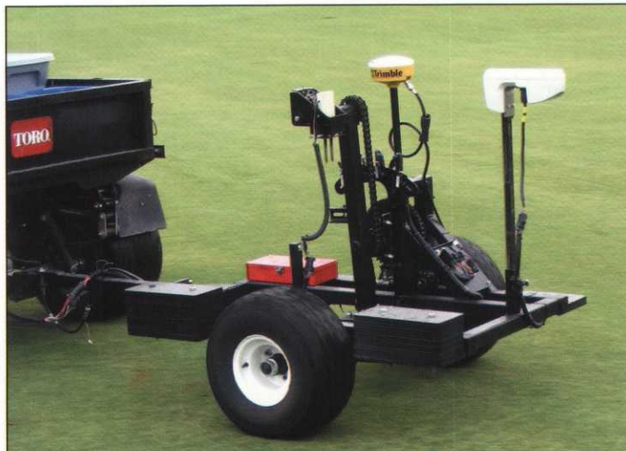
Figure 1. Mobile Sampling and Mapping Platform. Measures soil moisture, compaction, salinity, and plant reflectance while continually moving.
