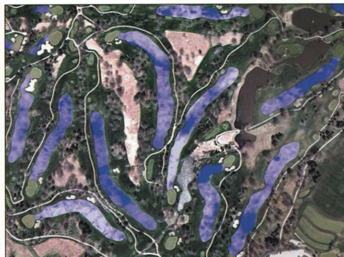
Figure 2. Soil moisture map for a portion of a golf course. The variability in soil moisture can be very dramatic. The darker the blue the higher the moisture content.
