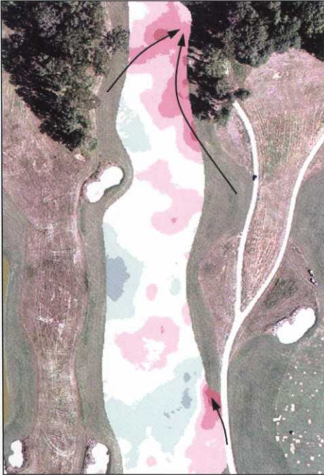
Figure 5. Compaction Management Map for a fairway with arrows representing the natural flow of cart traffic due to course design. Pinks represent higher compaction, white is average, and blues are lower compaction.
