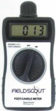
**Figure 3:** Instant (Hand-held) light meter. Great for collecting point in time measurements. (Spectrum Technologies)
