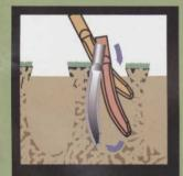
Our shatter knife technology - combined with our patented planetary motion - creates pore space throughout your root zone, eliminating compaction.
