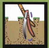
Our shatter knife technology - combined with our patented planetary motion - creates pore space throughout your root zone, eliminating compaction.
